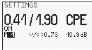
2 | By shortly pressing of the button ESC parameter to be changed are to be selected (inverted display) and to change by the buttons DOWN and UP. Unused memory locations can be displayed and disappear here with the parameter »ON« or »OFF«. Disappeared storage locations do not appear when switching on.
