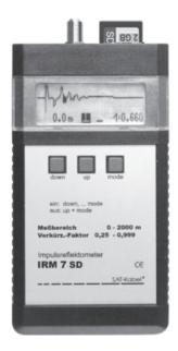
Pulse reflectometer with memory card
