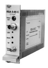
The **RSA** 5-65 **C** is a return path spectrum analyser. This analyser scans the signals of the return path in the spectrum 5–65 MHz. The signals are converted for a visual display in a PAL signal according the TV standard B/G. This procedure is patented. Thereby the return path signals from 5 to 65 MHz are displayed on the Y-axis with a grating of 5 MHz and on the X-axis the normalized level in  $dB(\mu V)$ .
